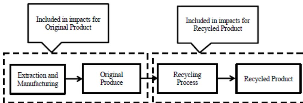
Figure 3: Recycling System Boundary
